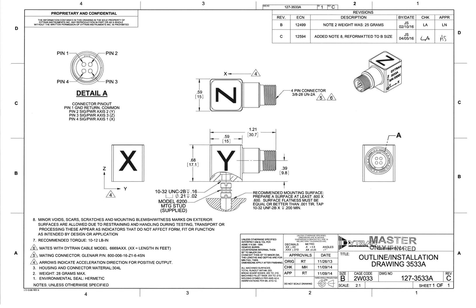
Doc No PERFORMANCE SPECIFICATION PS3533A 3533A Accelerometer, Triaxial, IEPE
