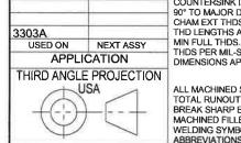
UNLESS OTHERWISE SPECIFIED UNLESS OTHERWISE SPECIFIED: INTERPRET DIM & TOL PER DIMENSIONS ARE IN INCHES. ASME Y14.5M - 1994. REMOVE BURRS. COUNTERSINK INTERNAL THDS 90° TO MAJOR DIA. CHAM EXT THDS 45° TO MINOR DIA. INCHES THD LENGTHS AND DEPTHS ARE FOR XX ± .03
