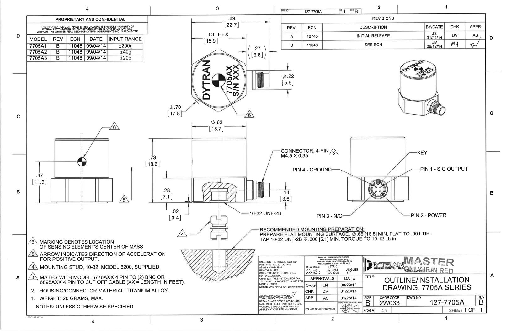
**Model Number** DOC NO PERFORMANCE SPECIFICATIONS 7705A3 PS7705A3 **DUAL ELEMENT ACCELEROMETER** REV C, ECN 11319, 09/22/14
