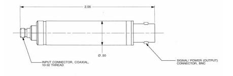
Units on the line drawing are in inches, units in brackets are in millimeters. Refer to 127-4705M4 for more information.
