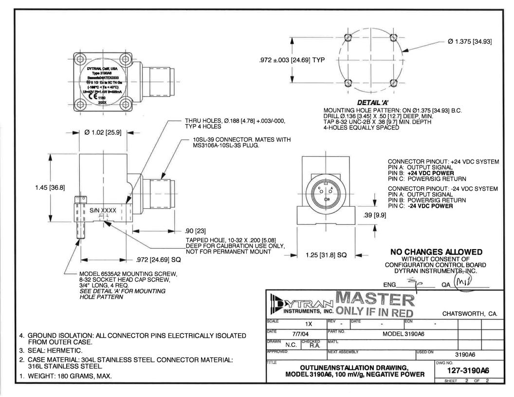
Model Number DOC NO PERFORMANCE SPECIFICATION PS3190A6 3190A6 SINGLE AXIS ACCELEROMETER REV B, ECN 15838, 07/13/20
