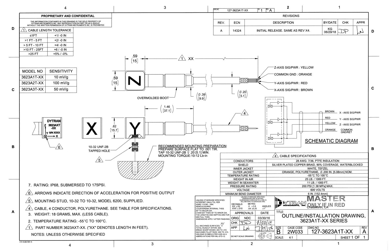
DOC NO. **Model Number** PERFORMANCE SPECIFICATION 3623A2T-XX PS3623A2T-XX TRIAXIAL IEPE ACCELEROMETER REV A, ECN 14324, 06/29/18
